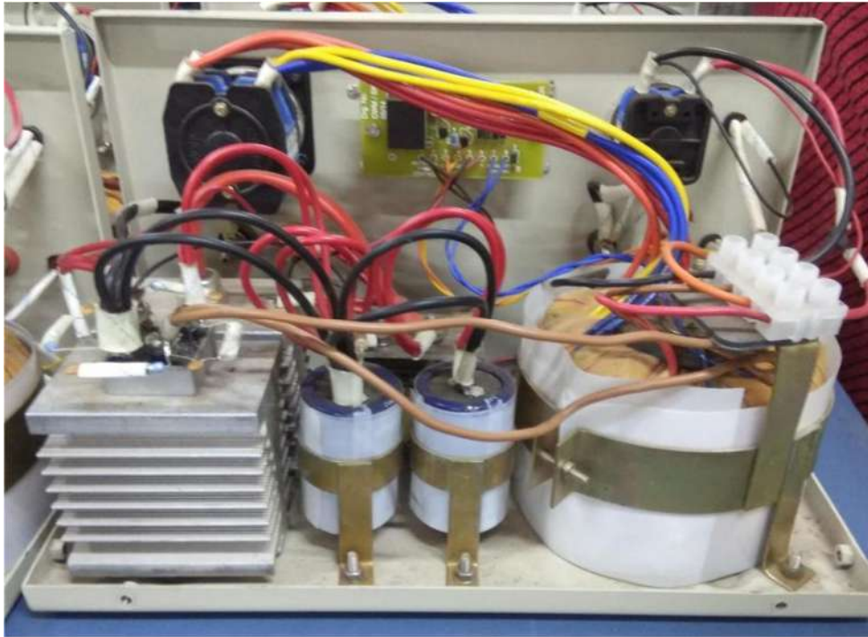
Fig. Track Feed Charger
