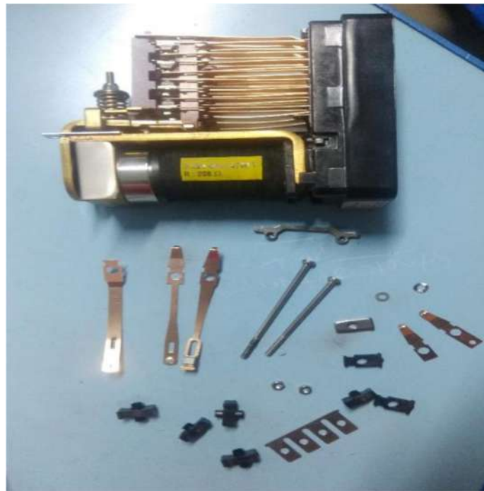
Fig. Relay and Its Components
